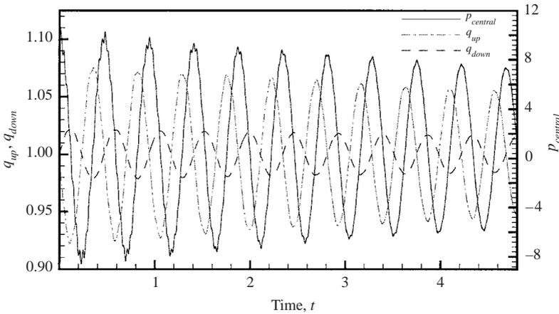
FIGURE 8. The pressure,  $p_{central}$ , at a central point in the fluid domain (at  $x = 4.81$ ,  $y = 0.39$ ) and the fluxes in the upstream and downstream rigid sections, respectively.  $p_{central}$  provides a measure of the pressure drops through the rigid sections.  $Re = 500$ ,  $T = 10^5$  and  $p_e = 1.40133$ .
