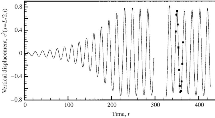
FIGURE 10. The vertical wall displacement at the centre of the membrane vs. time for  $Re = 450$ ,  $T = 10^2$  and  $p_e = p_e^{flush} = 0.96677$ . The two halves of the simulation were performed with different spatial resolutions. The symbols indicate the times at which the flow fields are documented in figure 12.
