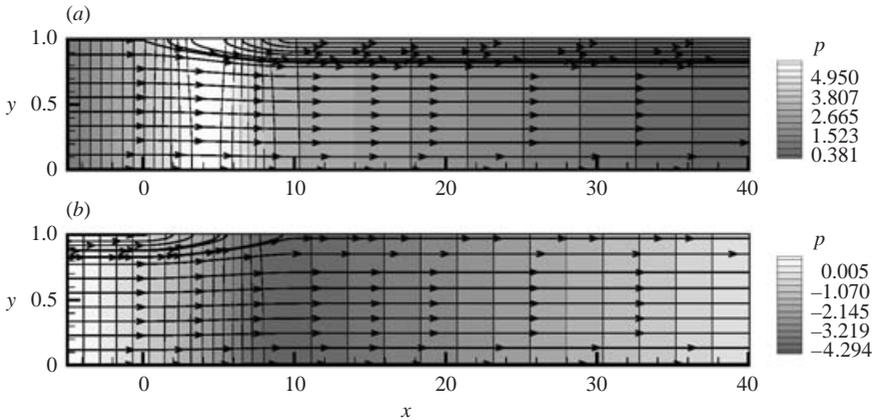
FIGURE 6. Pressure contours and instantaneous streamlines during the two characteristic phases of the small-amplitude oscillation. (a)  $t = 0.08$ , the wall moves inwards. (b)  $t = 0.32$ , the wall moves outwards.  $Re = 500$ ,  $T = 10^5$  and  $p_e = 1.40133$ .
