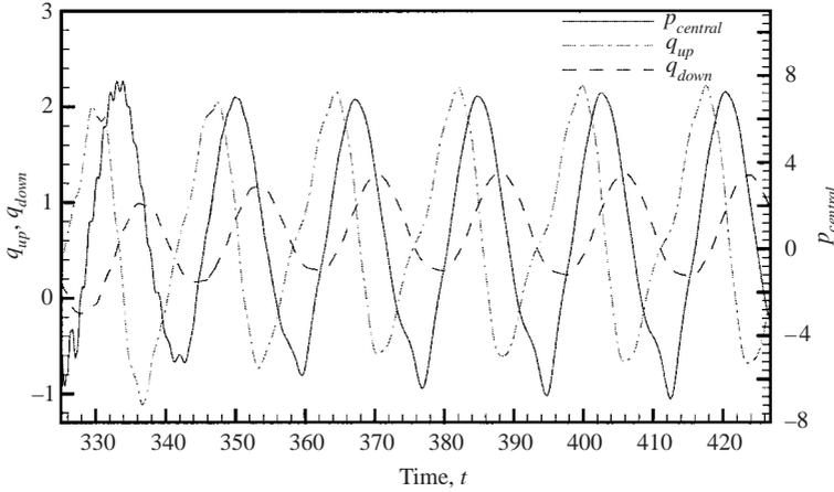
FIGURE 11. The pressure,  $p_{central}$ , at a nodal point in the elastic section and the fluxes  $q_{up}$  and  $q_{down}$  in the upstream and downstream rigid sections, respectively.  $Re = 450$ ,  $T = 10^2$  and  $p_e = p_e^{(flush)} = 0.96677$ . The pressure node is located on the line  $x = 4.93$  and moves vertically with the deforming mesh.
