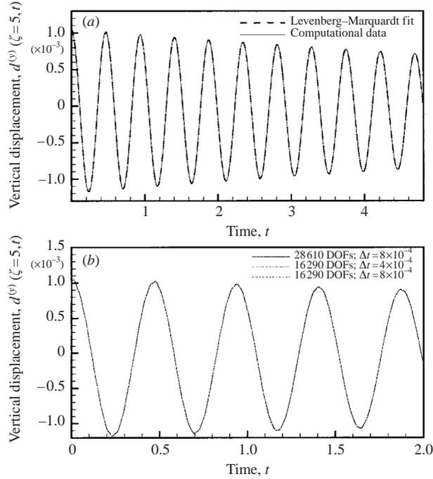
FIGURE 5. The vertical wall displacement at the centre of the elastic membrane vs. time for  $Re = 500$ ,  $T = 10^5$  and  $p_e = p_e^{(flush)} = 1.40133$ . The wall oscillates about the ‘flush’ position. (a) Comparison of the computational data (solid line) and the best fit to a damped harmonic oscillation (dashed line). (b) Results of the spatial and temporal convergence tests.
